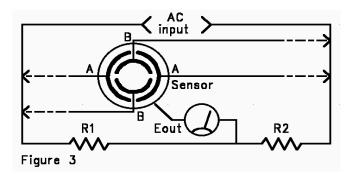
Caution! – Ensure that all test and operating circuits are entirely free of direct current. Direct current will cause level damage and/or instability.
