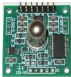
The Fredericks Company signal conditioning board with mounted TrueTilt metal dual-axis electrolytic tilt sensor
