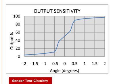
Tests were conducted by exciting the left and right electrodes with an AC signal of 400 Hz and an rms voltage to produce the maximum current at null as per operating specifications. Output readings are taken between the center electrode and the center of the balanced resistors R1 and R2. Tests were conducted at a temperature of  $+25^{\circ}$  C. See sensor test circuitry in figure 3. Output curve is shown in figure 1.
