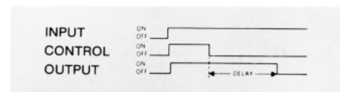
Apply input power. Upon application of control power, the output will energize. Remove control power and initiate delay period.
