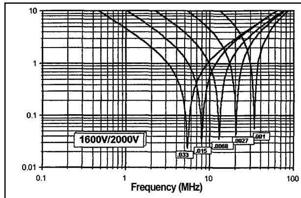
Please note: Capacitance values above are in  $\mu\text{F}$ . The resonant frequency and impedance shown above apply to units with a 0.250 lead length and are typical values only. Please contact us for data on the 100VDC rated units.
