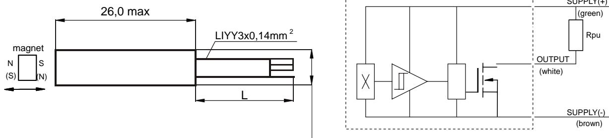
L – Length of wires depends on customer's requirement
