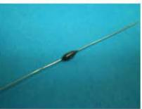
For ±1/10% (0.25%) resistance tolerance apply up to 50% of rated power to +85 Degrees Celsius.
